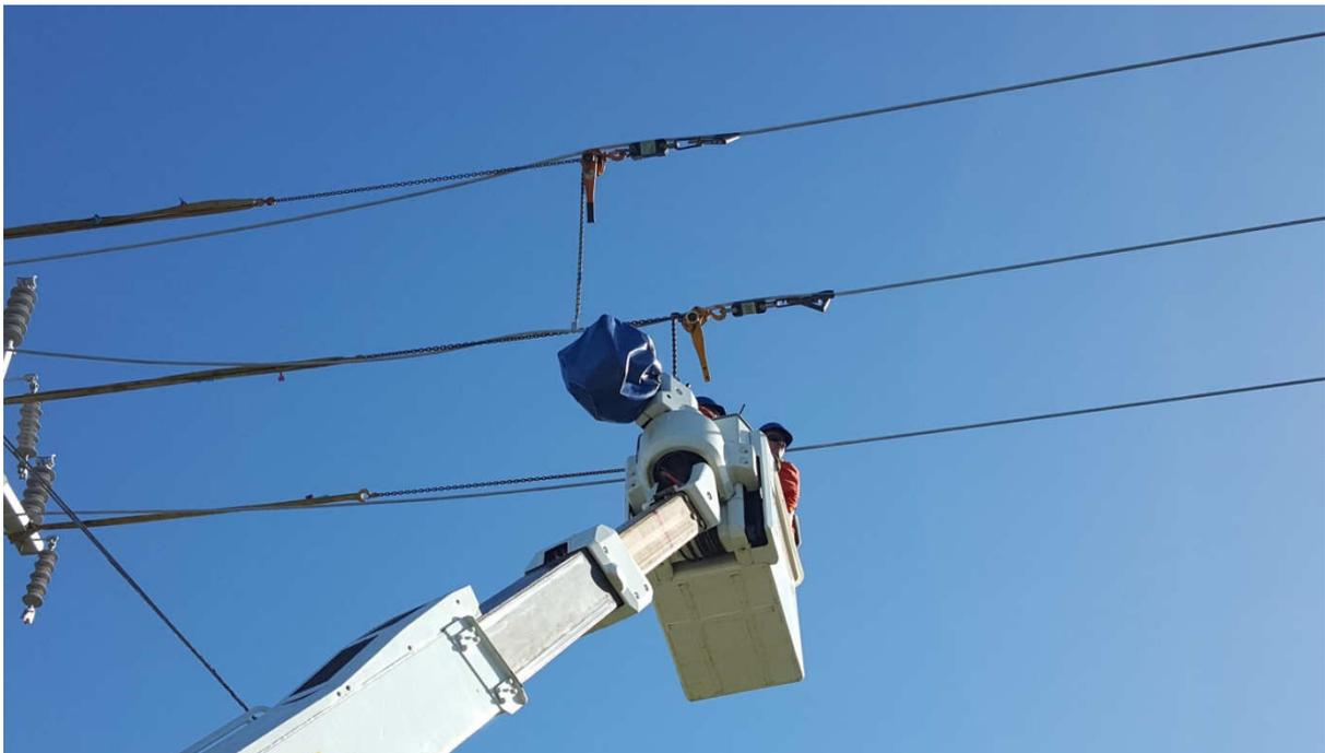
Figure 3: Dynamometers set up to measure tension
